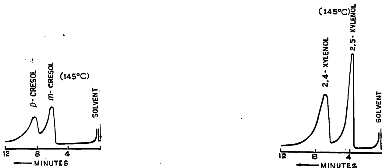
Fig. 1. Separation of m -cresol and p -cresol on a rubidium benzenesulphonate column.
